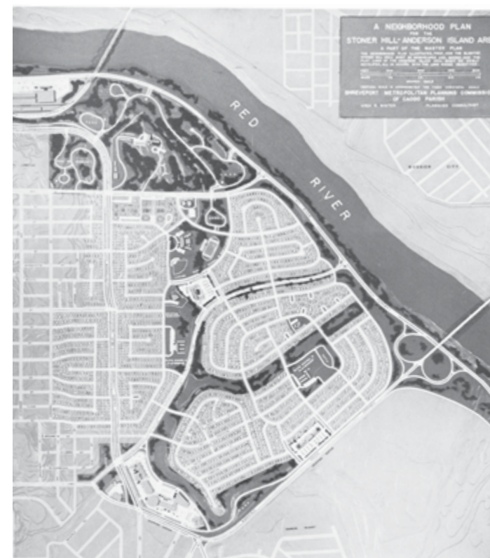
Conceptual plan illustrating redevelopment of the Stoner Hill - Anderson Island area from the 1956 Master Plan. Source: Shreveport-Caddo Metropolitan Planning Commission
